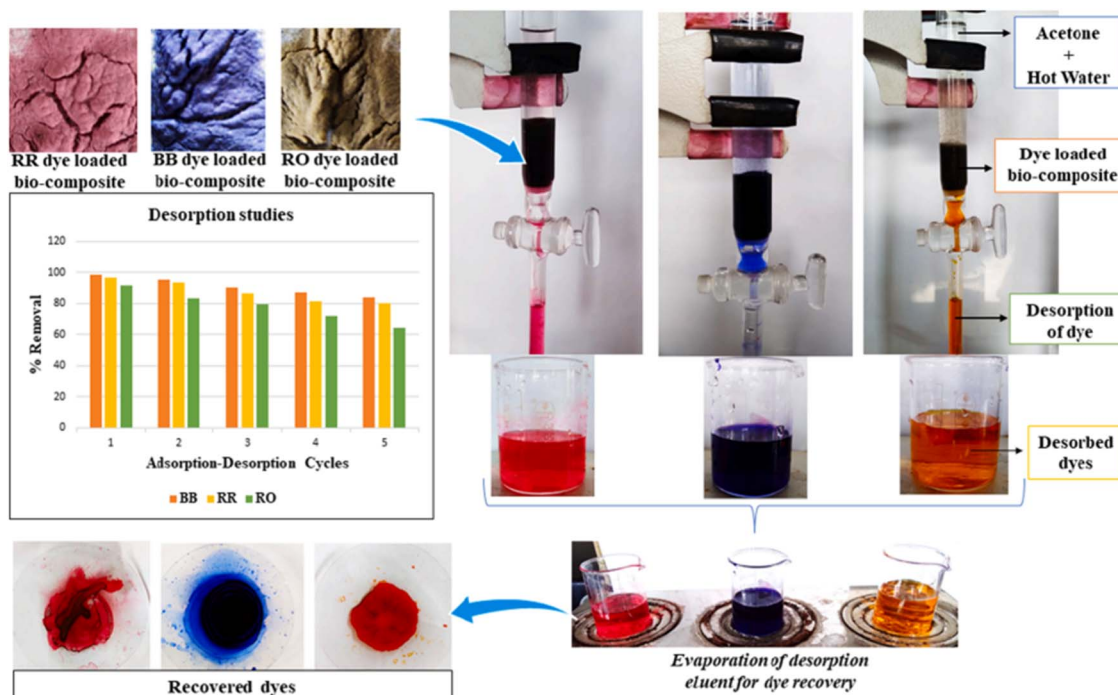
Fig. 7 Desorption studies of a dye-loaded bio-composite. 38
