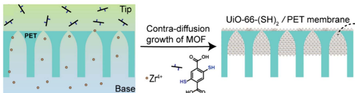
Fig. 18 (a) Schematic of ethylenediamine-modulated counter-diffusion. 204 Copyright 2016, American Chemical Society. (b) Engineering asymmetric sub-nanometer channels. 204 Copyright 2024, American Chemistry Society.
