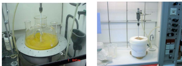
Fig. 1 High- and low-tech reactors for the synthesis of \text{IPr}\cdot\text{HCl} .
