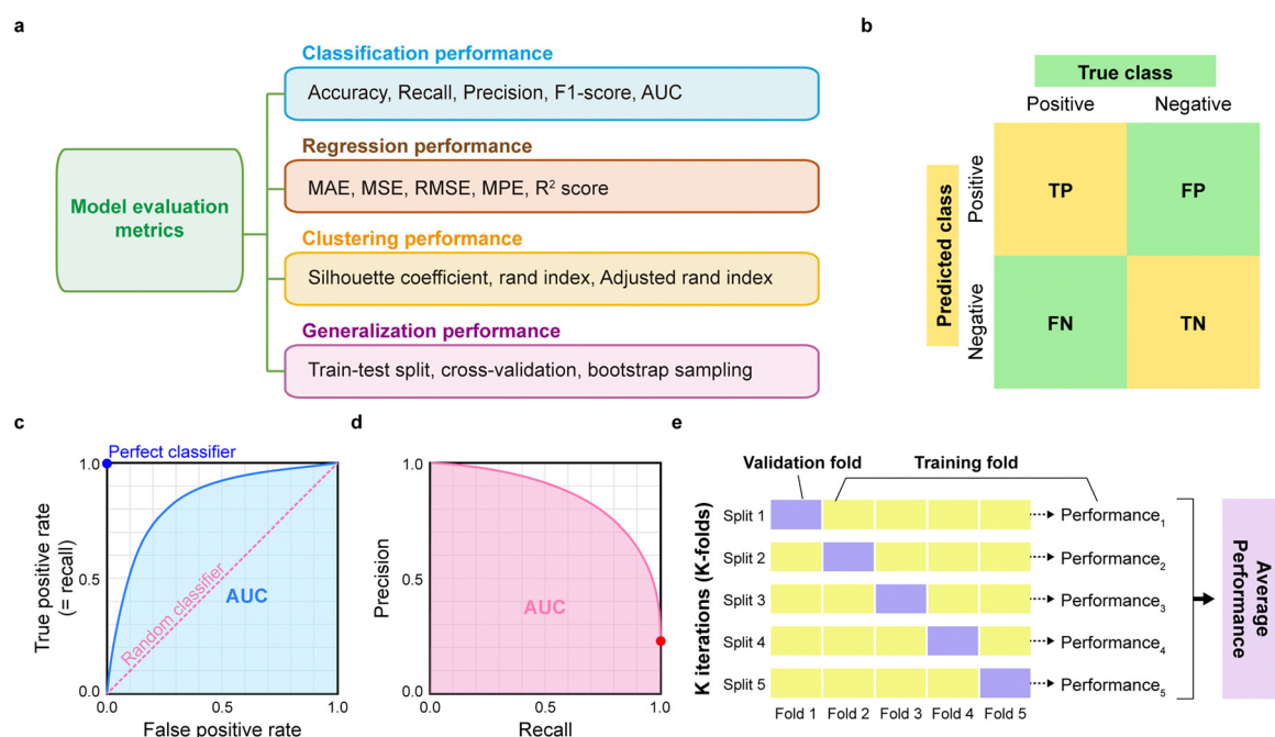
Fig. 6 Model evaluation metrics. (a) Categorization of model evaluation metrics. (b) Confusion matrix. (c) Receiver operating characteristic curve. (d) Precision–recall curve. (e) Schematic illustration of the K -fold cross-validation process.
