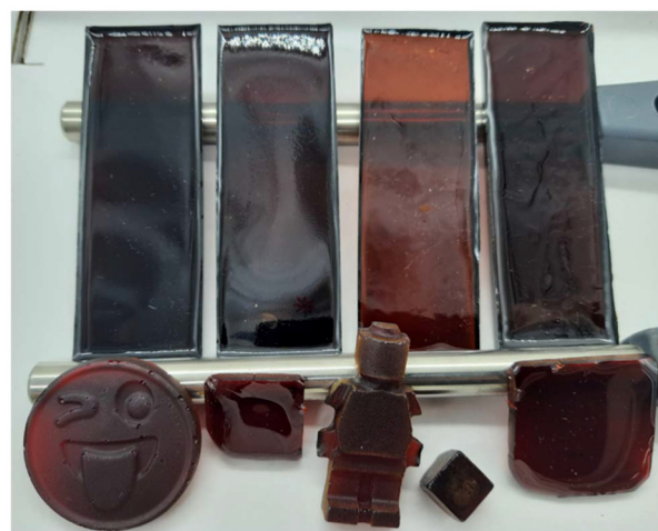
Fig. 8 Inverse vulcanised polymers that have been moulded into various shapes and dimensions, by pouring the pre-polymer into a mould and then curing the pre-polymer until it is shape persistent. Fully reacted inverse vulcanised polymers of low T_g can also be melt processed in this fashion.
