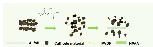
Fig. 1 Schematic illustration of the direct delamination of spent LiFePO 4 cathodes from the Al foil with the assistance of HPAA.
