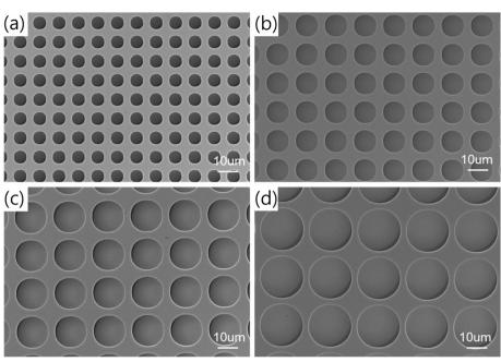
Fig. 3 SEM images of patterned holes. (a) Holes with a diameter of 5  $\mu$ m, (b) 10  $\mu$ m, (c) 15  $\mu$ m, and (d) 20  $\mu$ m are shown. The distance between patterns is 5  $\mu$ m, and the depth of all holes is 10  $\mu$ m. All scale bars are 10  $\mu$ m.
