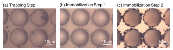
Fig. 4 Optical images of the particle immobilization step. (a) Represents the trapping step (b) represents the immobilization step using the capacitance effect, while (c) represents the immobilization step using a positive current, measured in a dried state. All scale bars are 10  $\mu$ m. The following are conditions of each step (a) 20  $V_{pp}$ , 1 MHz. (b) 20  $V_{pp}$ , 1 kHz. (c) 3  $V_{pp}$ , 1 MHz with a +3 V DC offset.
