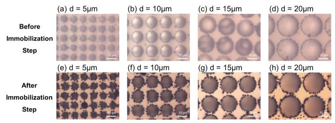
Fig. 5 Optical images of gold nanoparticles trapped along the edges of hole patterns. (a–d) Substrates before the immobilization step with hole pattern diameters of 5, 10, 15, and 20  $\mu$ m, respectively. The images were obtained using a covered, transparent ITO electrode. (e–h) Substrates after the immobilization step with diameters of 5, 10, 15, and 20  $\mu$ m, respectively, measured in a dried state. All scale bars are 10  $\mu$ m.
