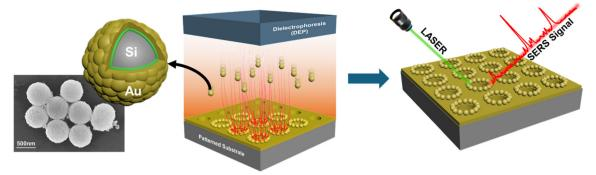
Fig. 1 Schematic illustration of the experimental process. Gold coated silica nanoparticles were arranged using dielectrophoresis (DEP), followed by SERS signal measurement through Raman spectroscopy.
