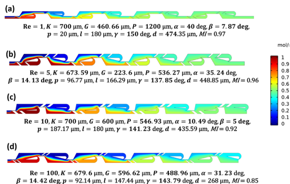
Fig. 10 Concentration profiles of Tesla micromixers modified with parallelogram barriers optimized using BO for different Re (a) Re = 1; (b) Re = 5; (c) Re = 10; (d) Re = 100.
