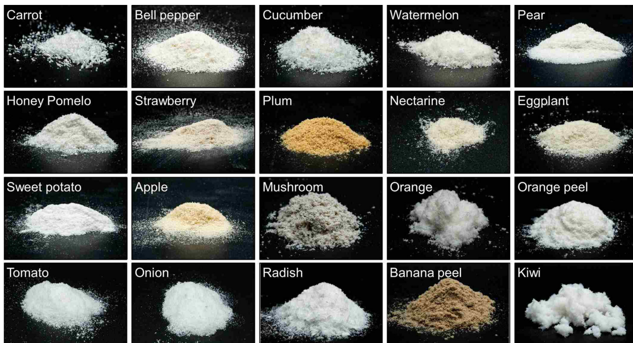
Fig. 2 Images of powders obtained after solvent exchange and sCO 2 -drying of various natural tissues. Respective sample names are given in the individual images.
