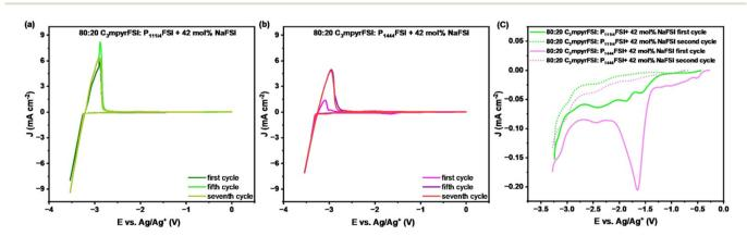
Fig. 3 Three-electrode cyclic voltammetry curves for mixed ILs. (a) C<sub>3</sub>mpyrFSI/P<sub>111i4</sub>FSI mixture, (b) C<sub>3</sub>mpyrFSI/P<sub>1444</sub>FSI mixture, (c) enlarged view of the first and second cycles prior to the onset of Na deposition.
