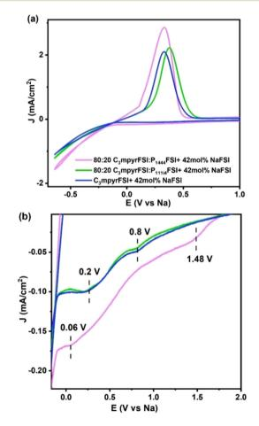
Fig. 2 (a) Cyclic voltammetry curves for the mixtures with 42 mol% NaFSI system at 1st cycle. (b) The enlarged reduction process.
