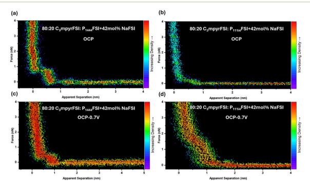
Fig. 6 Interfacial layering structure of mixed ILs through AFM force—distance two-dimensional histogram with probability colour bar on the right-hand. (a and b) at OCP; (c and d) at OCP-0.7V for C<sub>3</sub>mpyrFSI/P<sub>11114</sub>FSI mixture and C<sub>3</sub>mpyrFSI/P<sub>1444FSI</sub> mixture.
