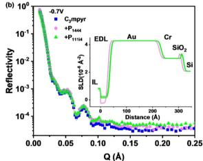
Fig. 5 Neutron reflectometry curves for electrolytes/electrode interfaces for (a) 0 V: (b) -0.7 V vs. OCP. Solid lines are fitting curves with four-slab model with varied parameters only for EDL. Insets are SLD profiles.
