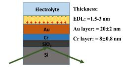
Fig. 10 Sketch of the NR experiment with approximate sizes of the lavers.
