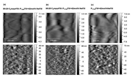
Fig. 7 Surface morphology of the formed solid interphase using ILs through AFM surface imaging at OCP -2.3 V for (a) C<sub>3</sub>mpyrFSI/P<sub>1114</sub>FSI mixture, (b) C<sub>3</sub>mpyrFSI/P<sub>1114</sub>FSI mixture and (c) P<sub>11114</sub>FSI + 42 mol% NaFSI.
