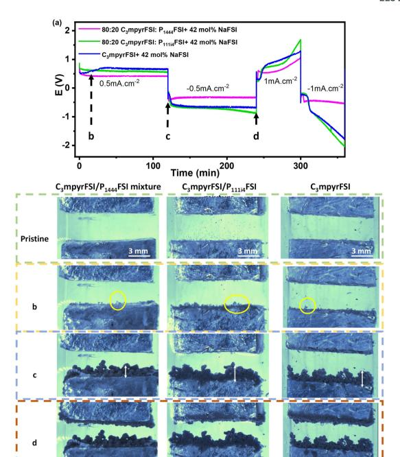
Fig. 8 In situ optical micrographs obtained for flooded optical cell cycled at 0.5 mA cm<sup>-2</sup>. (a) Cycling profile and morphology are shown at pristine; (b) after 10 min (Na deposition); (c) after first half-cycle; (d) after first cycle.
