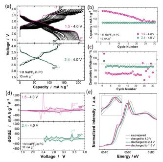
Fig. 2 (a) Charge/discharge curves, (b) capacity retention, (c) coulombic efficiency, and (d) differential capacity plots of P'2 Na<sub>2/3</sub>MnO<sub>2</sub> cycled with 1 M NaPF<sub>6</sub> in propylene carbonate (PC) electrolyte in the voltage ranges of  $1.5-4.0~\mathrm{V}$  and  $2.4-4.0~\mathrm{V}$  at a rate of  $10~\mathrm{mA~g}^{-1}$ . (e) Changes in Mn K-edge XAS spectra for P'2-Na<sub>2/3-v</sub>MnO<sub>2</sub> on electrochemical cycles.
