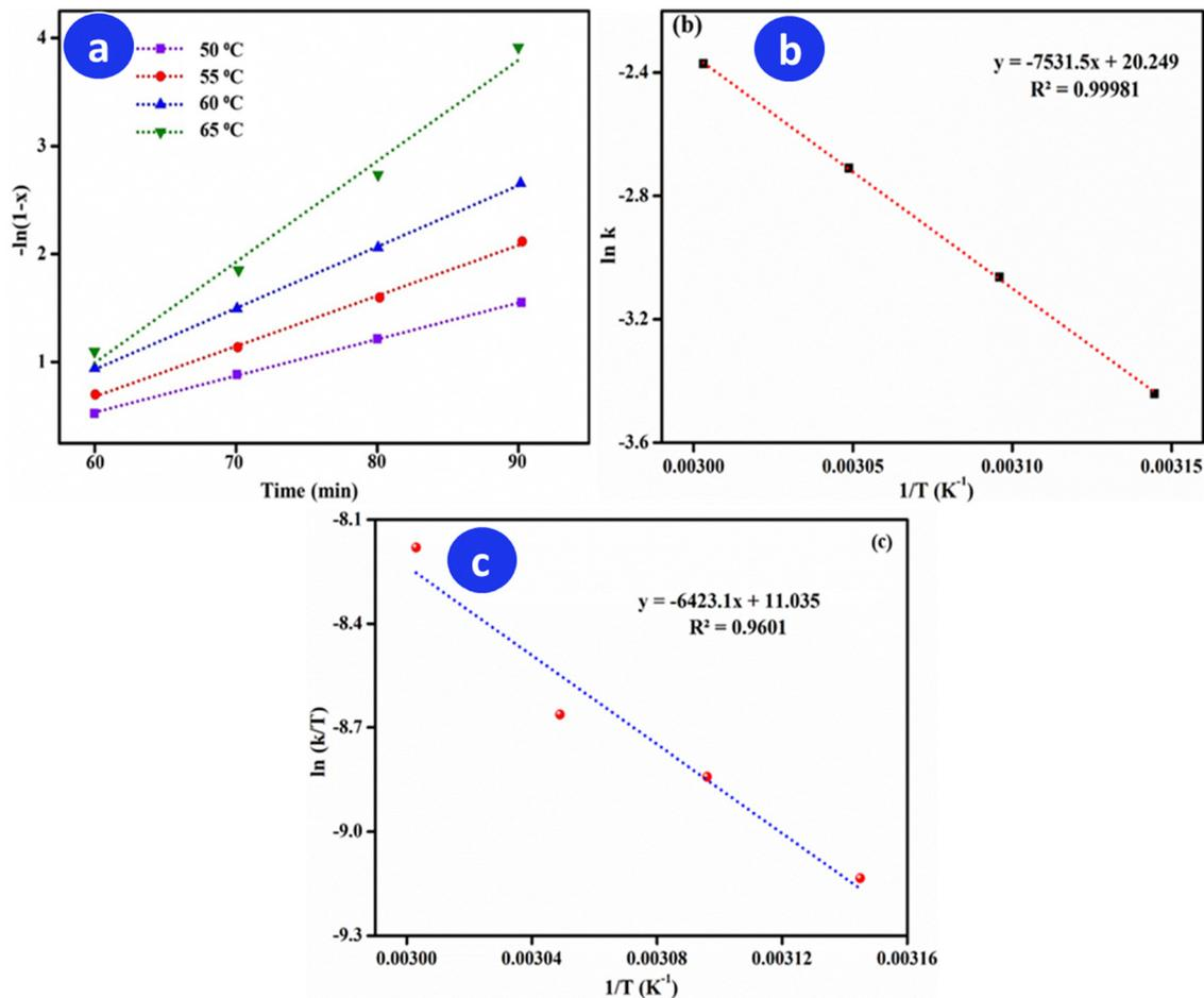
Fig. 4 (a) Plot of  $-\ln(1-X)$  vs. time, where  $X$  = glycerol conversion at different temperatures for acetalization reaction, (b) the corresponding Arrhenius plot of  $\ln k$  vs.  $1/T$ , and (c) thermodynamic behaviour of acetalization reaction.
