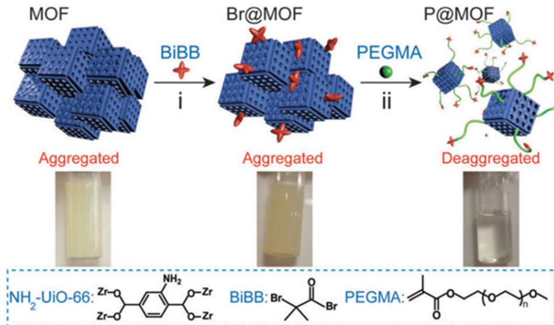
Fig. 2 Schematic illustration of ATRP on \text{NH}_2\text{-Uio-66} . The MOF particles transitioned from an aggregated state in aqueous solution to a well-dispersed state because of the growth of a hydrophilic polymer. Copyright 2015 Royal Society of Chemistry.
