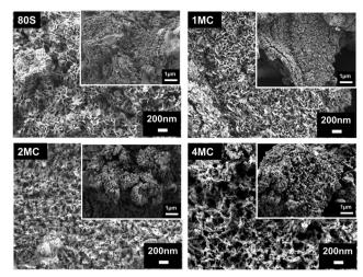
FESEM image of the MBGs surface after placing in SBF for 14 days The inset shows the same microstructure at a lower magnification.
