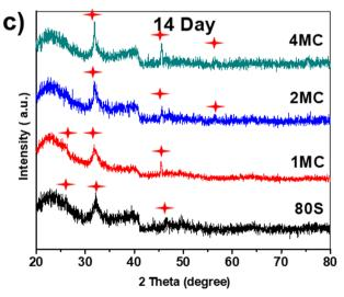
Fig. 8 XRD patterns of the investigated MBGs after placing them in SBF for (a) 1 day, (b) 7 days, and (c) 14 days; (formation of new hydroxyapatite phase marked by red stars).
