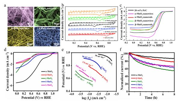
Fig. 3 The ORR performance and surface morphology of different MnO<sub>2</sub>. (a) SEM images of the samples obtained. (b) CV curves and (c) LSV curves of the obtained MnO<sub>2</sub> and 20 wt% Pt/C. Reproduced with permission.<sup>59</sup> Copyright 2019, Elsevier. (d) LSV curves, (e) Tafel slope and (f) chronoamperograms of MnO<sub>2</sub> with different crystal structures. Reproduced with permission.<sup>60</sup> Copyright 2023, Elsevier.
