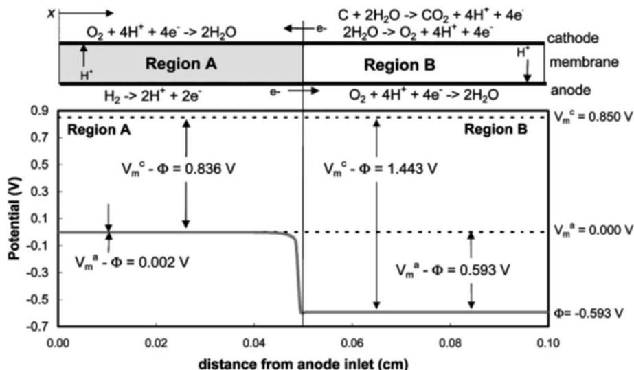
Fig. 1 Potential distributions along the anode flow path under reverse current conditions, where  $V_m^c$ ,  $V_m^a$  and  $\phi$  denote the potential of cathode metal, anode metal and electrolyte, respectively. Reproduced with permission.<sup>12</sup> Copyright 2005, The Electrochemical Society.
