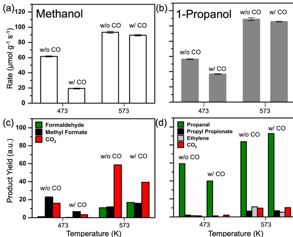
Fig. 3 The rate of (a) methanol and (b) 1-propanol oxidation in the absence (w/o CO) and presence (w/CO) of co-fed 2% CO at 473 K and 573 K over Pd<sub>3</sub>Au<sub>97</sub> RCT-SiO<sub>2</sub>, and the corresponding yield of products during (c) methanol and (d) 1-propanol oxidation. Reaction conditions: 4% 1-propanol, 10% O<sub>2</sub>, 0 or 2% CO, balanced in He; total flow rate = 50 mL min<sup>-1</sup>;  $m_{\text{cat}}$  = 10.0 mg.
