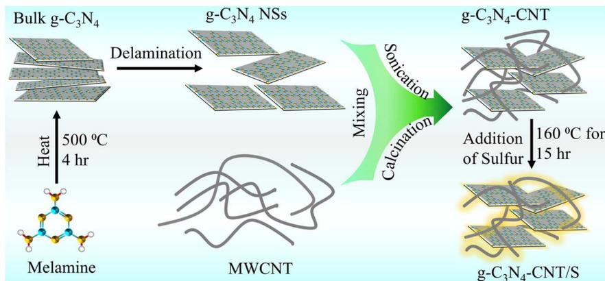
Scheme 1 Schematic illustration for the synthesis of the g-C<sub>3</sub>N<sub>4</sub>-CNT/S nanocomposite.
