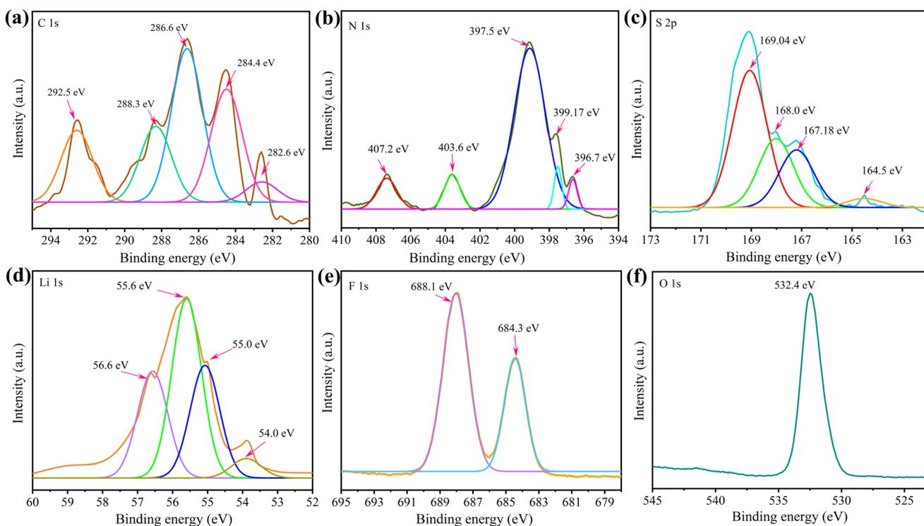
Fig. 8 (a-f) XPS spectra of the g-C<sub>3</sub>N<sub>4</sub>-CNT/S cathode obtained from the pouch cell cycled for 250 charge-discharge cycles.
