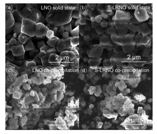
Fig. 9 SEM images of samples at 50 000× magnification (a) LNO prepared by solid state route (b) S-LRNO prepared by solid state route prepared by co-precipitation route (d) S-LRNO prepared by co-precipitation route.
