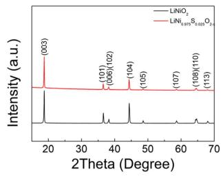
Fig. 1 XRD patterns of LiNiO<sub>2</sub> and S doped LiNiO<sub>2</sub> (solid state synthesis route)
