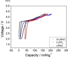
Fig. 6 (a) XRD patterns of  $Li_{1.1}Ni_{0.85}O_{2-x}$ , and  $Li_2SO_4$  ball milled  $Li_{1.1}$ - $Ni_{0.85}O_{2-x}$ . (b) Charge-discharge curves of solid state route synthesised LRNO, S-LRNO and LRNO with 5%Li<sub>2</sub>SO<sub>4</sub> between 2 and 4.3 V at 25 mA  $g^{-1}$  (after the formation cycle).
