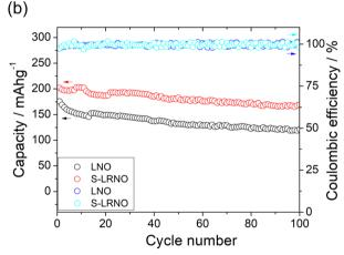
Fig. 5 (a) Initial charge–discharge curves of LNO and S-LRNO synthesised by the solid state method between 2 and 4.3 V at 25 mA  $\rm g^{-1}$  (after the formation cycle). (b) The cycling performance of LNO and S-LRNO at 25 mA  $\rm g^{-1}$ .
