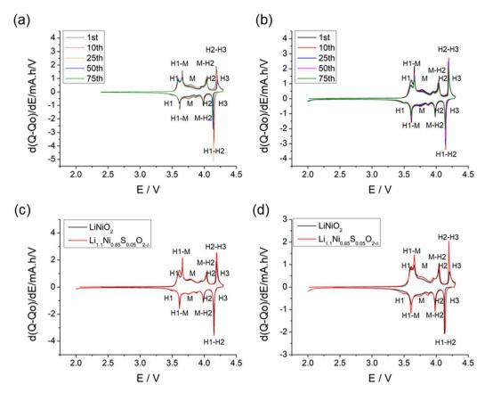
Fig. 10 dQ/dV curves of (a) LiNiO<sub>2</sub> and (b) Li<sub>1.1</sub>Ni<sub>0.85</sub>S<sub>0.05</sub>O<sub>2-x</sub> prepared through co-precipitation route; (c) comparison of LiNiO<sub>2</sub> and Li<sub>1.1</sub>Ni<sub>0.85</sub>S<sub>0.05</sub>O<sub>2-x</sub> at 1st cycle. (d) Comparison of LiNiO<sub>2</sub> and Li<sub>1.1</sub>Ni<sub>0.85</sub>S<sub>0.05</sub>O<sub>2-x</sub> at 75th cycle showing the clear preservation of H2-H3 transition in the latter.
