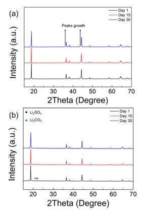
Fig. 4 XRD patterns of (a) LiNiO $_2$  and (b) Li $_{1.1}$ Ni $_{0.85}$ S $_{0.05}$ O $_{2-\delta}$  (solid state route) after the exposure in air after 1, 15 and 30 days.
