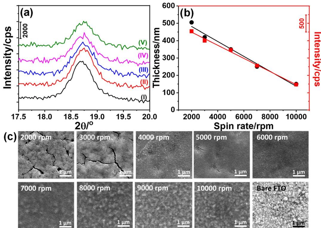
Fig. 1 (a) The XRD patterns of *m*-LMO-300-F# films between 17.5 and 20.0°,  $2\theta$ , coated at (I) 2000, (II) 3000, (III) 5000, (IV) 7000 and (V) 10 000 rpm, (b) the plots of the film thickness and X-ray intensity of the *m*-LMO-300-F# films versus spin-rate (black dots from SEM images and red squares are (111) diffraction line intensity values at 18.7°,  $2\theta$ ), and (c) the SEM images (top view) of the thin films at indicated spin-rates.
