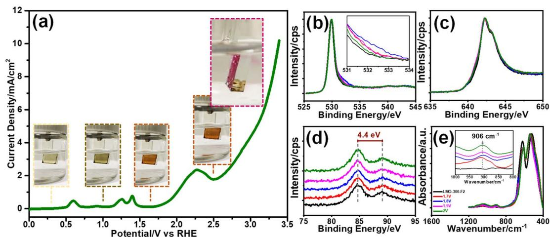
Fig. 4 (a) The LSV curve of the *m*-LMO-300-F2 electrode between −0.05 and 3.4 V in 1.0 M LiNO<sub>3</sub> with a 5 mV s<sup>−1</sup> scan rate (insets: color of the electrodes at indicated potentials) and the XPS spectra of *m*-LMO-300-F2 at various potentials in the (b) O 1s, (c) Mn 2p, and (d) Mn 3s regions, where black: 1.6 V, red: 1.7 V, blue: 1.8 V, pink: 1.9 V, and green: 2.0 V. (e) The FTIR spectra of *m*-LMO-300-F2 at various potentials.
