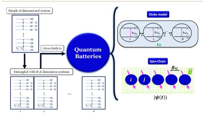
Fig. 11 Quantum battery sum-up schematics.
