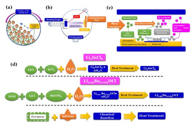
Fig. 5 Synthesis methods: (a) high energy density ball milling;<sup>76</sup> (b) pulsed laser deposition (PLD);<sup>77</sup> (c) chemical vapor deposition (CVD);<sup>78</sup> (d) water mediated synthesis of Li<sub>3</sub>InCl<sub>6</sub>, <sup>41</sup> Li<sub>2,99</sub>Ba<sub>0,005</sub>OCl, <sup>29</sup> K<sub>2,99</sub>Ba<sub>0,005</sub>OCl and Na<sub>2,99</sub>Ba<sub>0,005</sub>OCl. <sup>28</sup>
