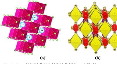
Antiperovskite electrolytes structures: (a) Li<sub>3</sub>OCl;<sup>29</sup> (b) Li<sub>6</sub>SO(BH<sub>4</sub>)<sub>2</sub>,<sup>91</sup> CIF files: ref. 53–66
