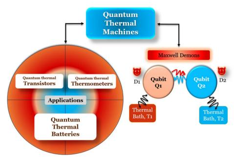
Fig. 15 Quantum feedback thermal machines and their applications. Qubits  $Q_1$  and  $Q_2$  are monitored by  $D_1$  and  $D_2$ , connected to thermal baths  $T_1$  and  $T_2$ . In the case of Maxwell's demons,  $T_1 = T_2 = T$ . The two baths can also have different temperatures <sup>148</sup> and work as refrigerators.
