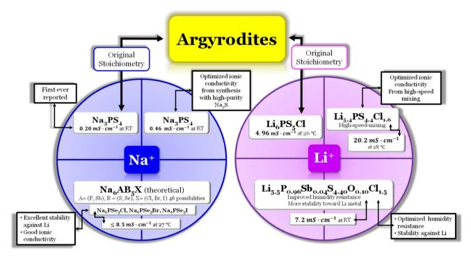
Fig. 6 Argyrodite summary scheme,  $\text{Li}_6\text{PS}_5\text{Cl}$ ;  $^{14}\text{Li}_{5.4}\text{PS}_{4.4}\text{Cl}_{16}$ ;  $^{30}\text{Li}_{5.5}\text{P}_{0.96}\text{Sb}_{0.04}\text{S}_{4.40}\text{O}_{0.10}\text{Cl}_{1.5}$ ;  $^{83}\text{Na}_3\text{PS}_4$ ;  $^{84.85}$  and  $\text{Na}_6\text{AB}_5\text{X}$ , A = (P, Sb),  $\text{B} = =(\text{S, Arg}_5)$ ;  $\text{Na}_3\text{PS}_4$ ; Se), and  $X = (Cl, Br, I).^{86}$
