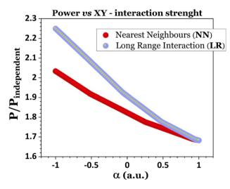
**Fig. 14** Charging power of a spin-chain quantum battery as a function of the anisotropy factor: N=4 and B=3 a.u.,  $\omega=4B$ , g=B and p=1.
