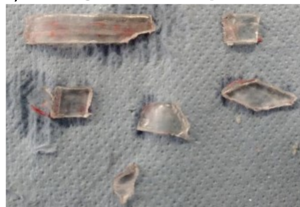
Fig. 6 Release of silver from PC by dissolution of the separation layer. (a) Shredded fragments of PC with large silver tracks on PVA layer. (b) Fragments after separation of silver by dissolution of PVA using water at ambient temperature.
