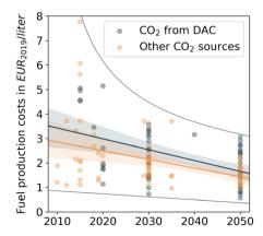
Fig. 3 Fuel production costs from literature review for CO<sub>2</sub> provision from DAC and other CO<sub>2</sub> sources. The depicted regression line of all 113 data points (with a 95% confidence interval shading) has an adjusted  $R^2$  value of 0.23 (0.13) for  $CO_2$  from DAC (other sources), revealing the high spread in the data.
