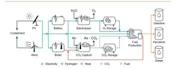
Fig. 5 PtL-SAF production process flowchart including all modelled components and energy/mass streams. "Fuel production" includes a reverse water-gas shift reaction step, Fischer-Tropsch synthesis, and refining.
