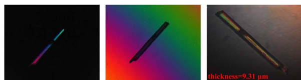
Fig. 5 Experimental birefringence at 546 nm for \text{Pb}_2(\text{SeO}_3)(\text{SiF}_6) .
