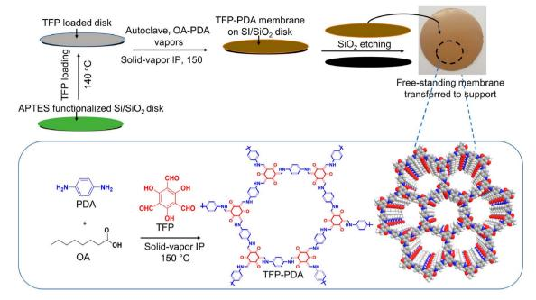
Fig. 2 Scheme of solid-vapor interfacial polymerisation (IP) for the 1,3,5-triformylphloroglucinol-polyamide (TFP-PDA) membrane, including membrane growth and HF etching step to obtain a free-standing membrane. Digital photos of the TFP-PDA membrane and the molecular reaction are presented. Copyright 2020 American Chemical Society.
