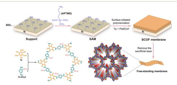
Fig. 5 Schematic route for the preparation of the SCOF membrane grafted on silicon wafers and the free-standing SCOF membrane, molecular structures of Tp, Pa-SO<sub>3</sub>H and TpPa-SO<sub>3</sub>H. Copyright 2021 Wiley-VCH GmbH.
