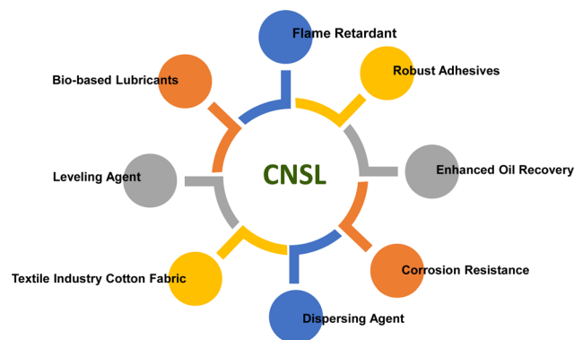
Fig. 13 Different key applications of CNSL derivatives in various industries.
