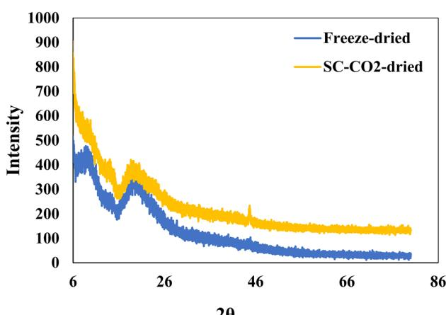
Fig. 3 XRD patterns of freeze-dried and SC-CO<sub>2</sub>-dried sorghum protein powders.
