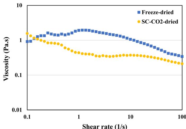
Fig. 7 Viscosity of freeze-dried and SC-CO<sub>2</sub>-dried sorghum proteins at 20 °C with a pH of 12.
