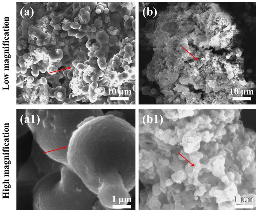
Fig. 2 SEM images of (a) and (a1) freeze-dried sorghum proteins, and (b) and (b1) SC-CO<sub>2</sub>-dried sorghum proteins.
