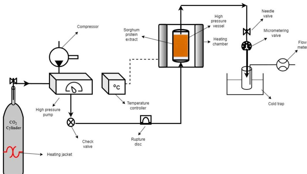
Fig. 1 Schematic diagram of the SC-CO<sub>2</sub> drying system.
