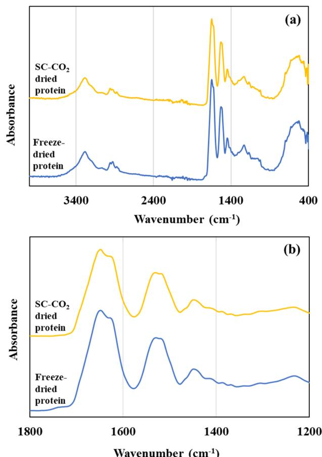
Fig. 5 (a) FTIR spectra of SC-CO<sub>2</sub>-dried and freeze-dried sorghum proteins, and (b) FTIR spectra of the samples focusing on the amide I and amide II regions.
