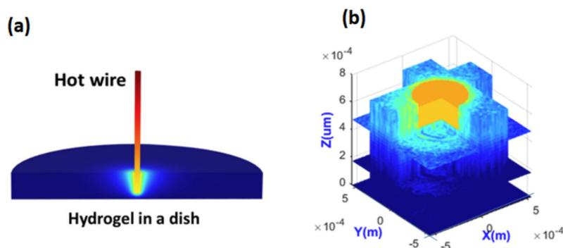
**Fig. 8** Ultrabright fluorescent nanothermometers- nanoparticles allow measuring 3D mapping of temperature distribution. (a) 3D temperature distribution of a heated wire in hydrogel simulated with a stationary numerical model solution. (b) 3D temperature measurements using nano-UMSP. [Reproduced from ref. 30 with permission from RCS, copyright 2021].
