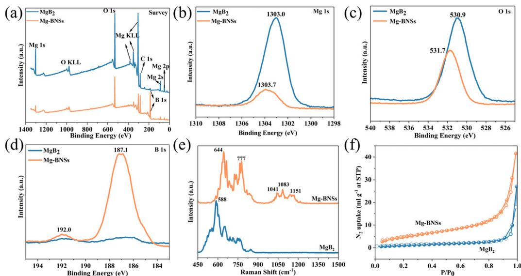
**Fig. 2** XPS spectra of (a) survey, (b) Mg 1s, (c) O 1s, and (d) B 1s of MgB<sub>2</sub> and Mg-BNSs. (e) Raman spectra of MgB<sub>2</sub> and Mg-BNSs. (f) N<sub>2</sub> adsorption-desorption curves of MgB<sub>2</sub> and Mg-BNSs.
