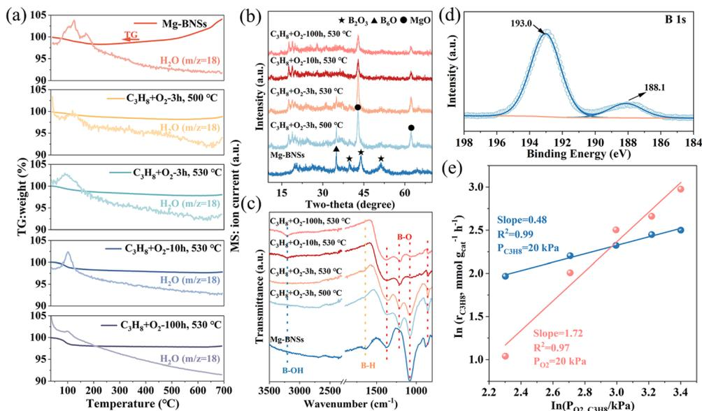
**Fig. 4** (a) TG-MS analysis of Mg-BNSs and their spent forms under an O<sub>2</sub>-rich atmosphere (20% O<sub>2</sub> + 80% N<sub>2</sub>). (b) XRD patterns and (c) FT-IR spectra of Mg-BNSs and the spent Mg-BNSs activated in the reaction atmosphere at different temperatures and durations. (d) B 1s XPS spectrum of Mg-BNSs tested for 100 h over ODHP. (e) Reaction rate as a function of the partial pressure of propane and oxygen in ODHP over Mg-BNSs. The data were obtained at 480 °C.
