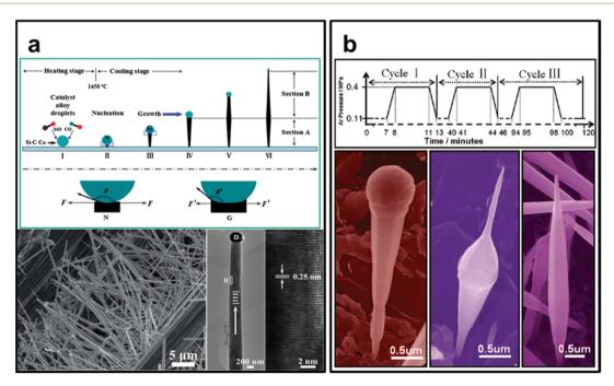
Fig. 7 (a) Controlled growth of quasialigned SiC nanoarrays with clear and sharp tips. Reprinted with permission from ref. 125. Copyright 2014 by Royal Society of Chemistry; (b) manipulate and control the morphology of SiC nanowires by varying the pressure of the source species. Reprinted with permission from ref. 126. Copyright 2008 by Royal Society of Chemistry.
