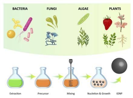
Biosynthesis of IONzymes using different green sources
