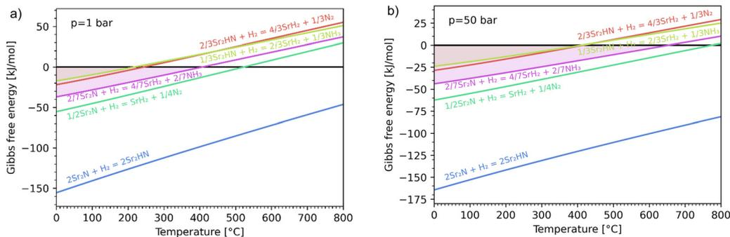
Fig. 4 Ellingham diagram of the hydrogenation step for the reactions (7)–(11). Variation of the Gibbs free energy change per mol H<sub>2</sub> as a function of temperature for: (a) standard  $\Delta G_{\text{rxn}}^\circ$ ; and (b)  $\Delta G_{\text{rxn}}$  at 50 bar assuming 20% reaction extent.
