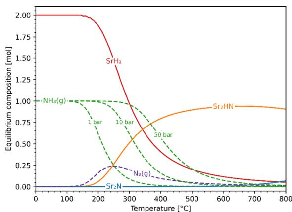
Fig. 5 Equilibrium composition of the Sr–H–N system as a function of temperature at 1 bar with initial conditions Sr<sub>2</sub>N + 10H<sub>2</sub>. Also shown are the NH<sub>3</sub> curves at 10 and 50 bar. Solid lines: solid phases; dashed lines: gaseous phases.
