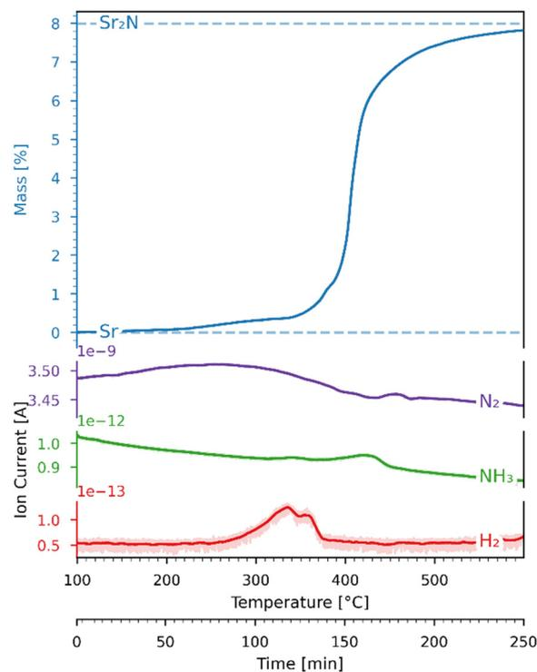
Fig. 6 Variations of mass (recorded by the TGA) and ion current (recorded by the mass spectrometer) as a function of time and temperature for the Sr-nitridation under 100% N<sub>2</sub>. Blue dashed lines: theoretical mass changes for no conversion (0%) and full conversion to Sr<sub>2</sub>N (7.99%) according to reaction (3). The ion current signals correspond to N<sub>2</sub> (purple), NH<sub>3</sub> (green), and H<sub>2</sub> (red).
