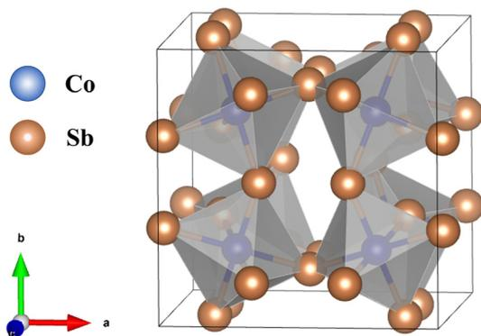
**Fig. 11** Illustration of the crystal structure of the  $\text{CoSb}_3$ -based alloy, which crystallizes into octahedrons within the space group  $Im\bar{3}$ . The structure is characterized by a void at the center of the cubic lattice. Crystal structure information was sourced from materialproject.org and visually represented using VESTA.<sup>48</sup>
