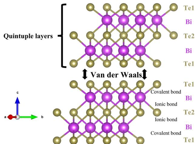
Fig. 10 Bi<sub>2</sub>Te<sub>3</sub> exhibits a rhombohedral structure consisting of quintuple layers, Te1–Bi–Te2–Bi–Te1, connected by van der Waals bonding along the *c*-axis. Information on the crystal structure was sourced from materi-alproject.org and visually represented using VESTA.<sup>48</sup>
