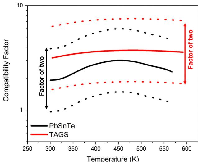
Fig. 9 The compatibility factors of TAGS<sup>37</sup> and PbSnTe<sup>47</sup> in the p-type legs of the multi-mission radioisotope thermoelectric generator (MMRTG). The bold and dotted lines represent the compatibility factors calculated based on eqn (3) and the compatible range of a factor of two, respectively.
