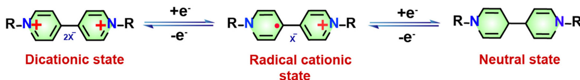
Scheme 1 Schematic representation of different redox states of a viologen moiety. The viologen moiety undergoes two reversible reduction reactions. The dicationic state of the viologen moiety is the most stable state of viologen. [R = alkyl/aromatic].
