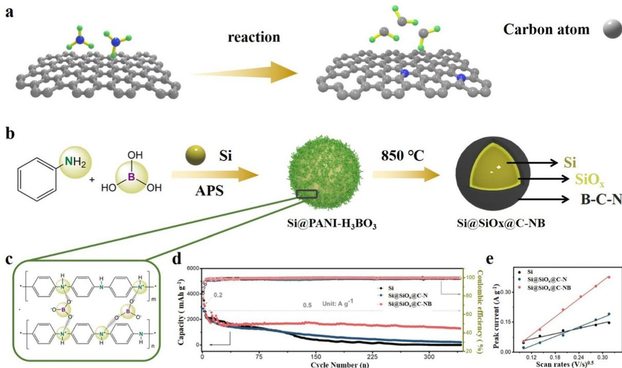
Fig. 9 (a) Schematic diagram of doping manufacturing defects. (b) Synthetic approach of Si@SiO<sub>x</sub>@C-NB, (c) polymer molecular structure, (d) cycling stability for 340 cycles at 0.5 A g<sup>-1</sup> and (e) linear fits for varying sweeping rate CV profiles.<sup>89</sup> Reproduced from ref. 89 with permission from John Wiley and Sons, Copyright 2022.
