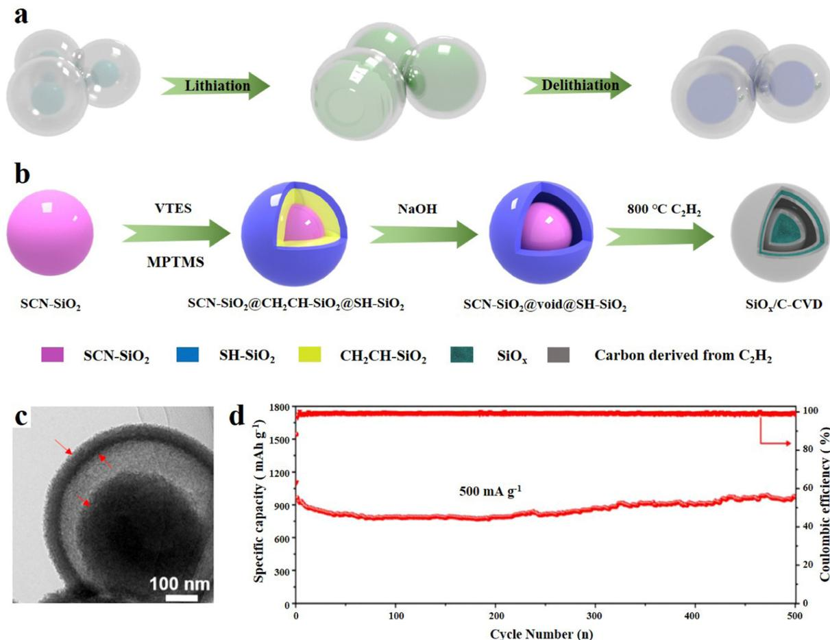
Fig. 6 (a) The evolution of the yolk@shell structure during lithiation/delithiation. (b) Schematic illustration of the preparation of SiO<sub>x</sub>/C-CVD, (c) TEM image and (d) long-term cycling performance at 500 mA g<sup>-1</sup>.<sup>98</sup> Reproduced from ref. 98 with permission from Elsevier, Copyright 2019.
