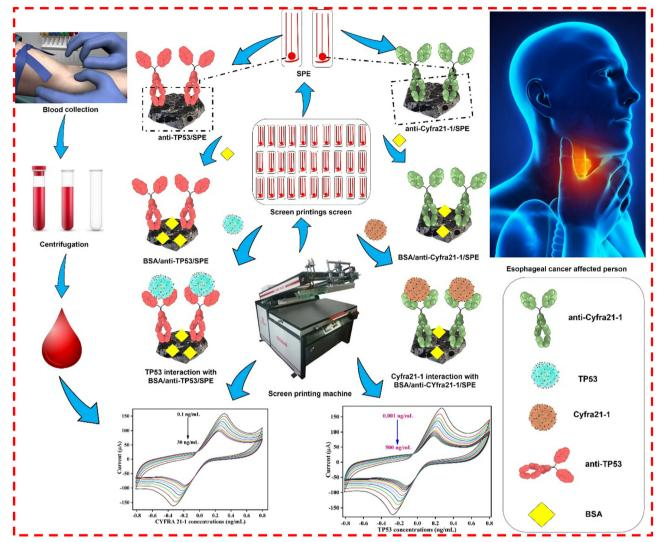
Scheme 1 The fabrication of SPE and the development of two immunoplatforms, i.e., BSA/anti-CYFRA21-1/SPE and BSA/anti-TP53/SPE for the dual detection of CYFRA21-1 and TP53 cancer biomarkers, respectively, in the serum samples of esophageal-affected cancer patients.
