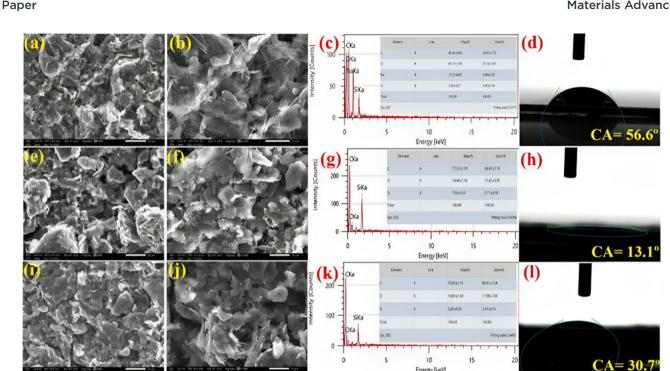
Fig. 3 SEM images of the SPE at (a) low (20 μm) and (b) high (10 μm) magnification; (c) EDS, and (d) CA. SEM images of anti-CYFRA21-1/SPE at (e) low (20 μm) and (f) high (10  $\mu$ m) magnifications; (g) EDS and (h) CA. SEM images of anti-TP53/SPE at (i) low (20  $\mu$ m) and (j) high (10  $\mu$ m) magnifications; (k) EDS and (l) CA.
