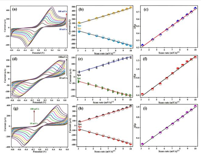
Fig. 5 Scan rate analysis of different electrodes: (a) SPE, (d) BSA/anti-CYFRA21-1/SPE, and (g) BSA/anti-TP53/SPE in PBS.  $I_{pa}$  and  $I_{pc}$  peak current curves of (b) SPE, (e) BSA CYFRA21-1/SPE and (h) BSA/anti-TP53/SPE electrodes, respectively, with the square root of scan rates. Changes in peak potential ( $\Delta E_{\rm p}$ ) versus the square root of scan rates for (c) SPE, (f) BSA/CYFRA21-1/SPE and (i) BSA/anti-TP53/SPE bioelectrodes, respectively
