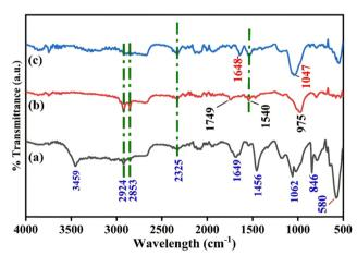
Fig. 2 FTIR analysis of different electrodes: (a) SPE, (b) anti-CYFRA21-1/ SPE, and (c) anti-TP53/SPE immunoplatforms.
