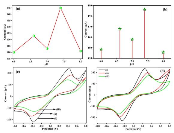
Fig. 4 A pH study of (a) BSA/anti-CYFRA21-1/SPE and (b) BSA/anti-TP53/SPE immunoelectrodes, (c) CV curves of (i) SPE, (ii) anti-CYFRA21-1/SPE, (iii) BSA/anti-CYFRA21-1/SPE and (d) CV curves of (i) SPE, (ii) anti-TP53/SPE (iii) BSA/anti-TP53/SPE immunosensors in PBS.
