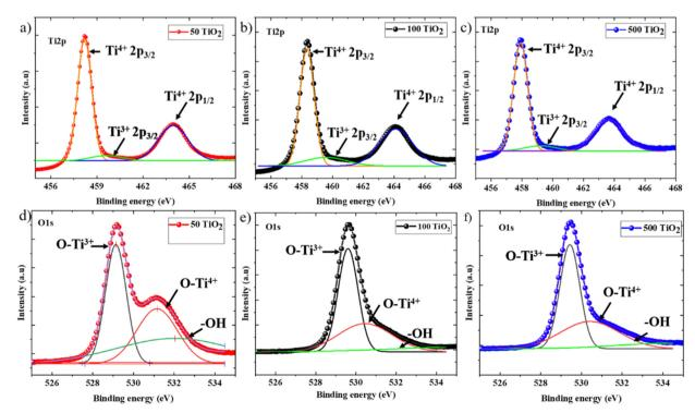
Fig. 6 (a)-(c) Ti2p XPS spectra and (d)-(f) O1s XPS spectra of 50 TiO2, 100 TiO2 and 500 TiO2.
