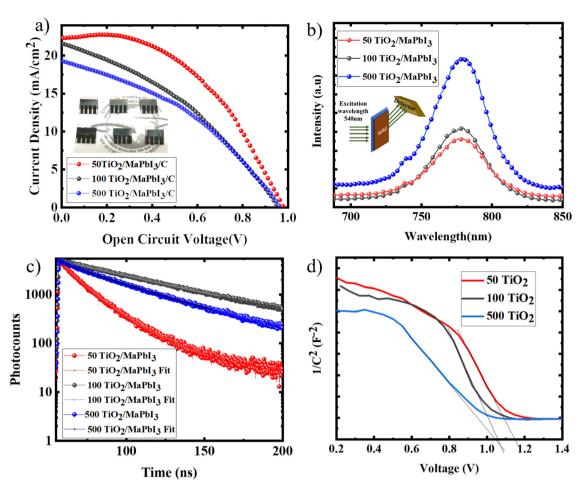
Fig. 7 (a) IV characteristics of CPSCs with 50 TiO2, 100 TiO2 and 500 sintered TiO2 as the ETL; (b) PL spectra and (c) TRPL spectra of MaPbI3 films deposited on 50 TiO2, 100 TiO2 and 500 sintered TiO2. (d) Mott-Schottky analysis at 1 kHz for the TiO2/MaPbI3 carbon heterojunction solar cell.
