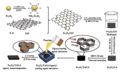
Fig. 11 The schematic for the fabrication of the Fe<sub>3</sub>O<sub>4</sub>/TAGA/epoxy nanocomposites; reproduced with permission from ref. 104, copyright reserved Elsevier 2019
