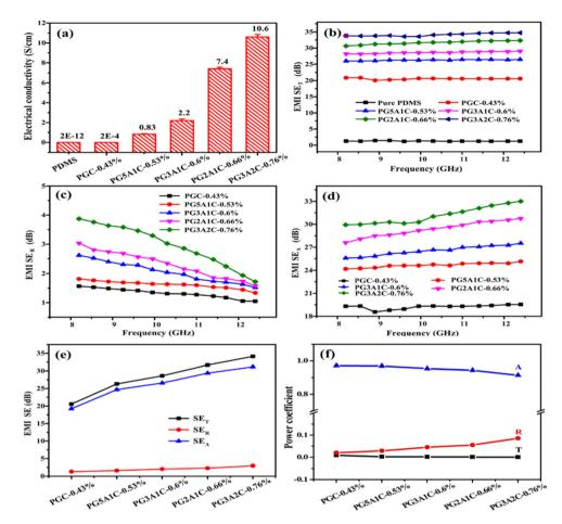
Fig. 10 (a) Electrical conductivity and (b) SE<sub>T</sub> of PDMS, PGC-0.43% and PGACs in the X-band, (c) SE<sub>R</sub>, (d) SE<sub>A</sub>, (e) the average SE<sub>T</sub>, SE<sub>R</sub>, SE<sub>A</sub>, and (f) the average power coefficients (A, R, T) of PGC-0.43% and PGACs in the X-band; reproduced with permission from ref. 94, copyright reserved Elsevier 2019.
