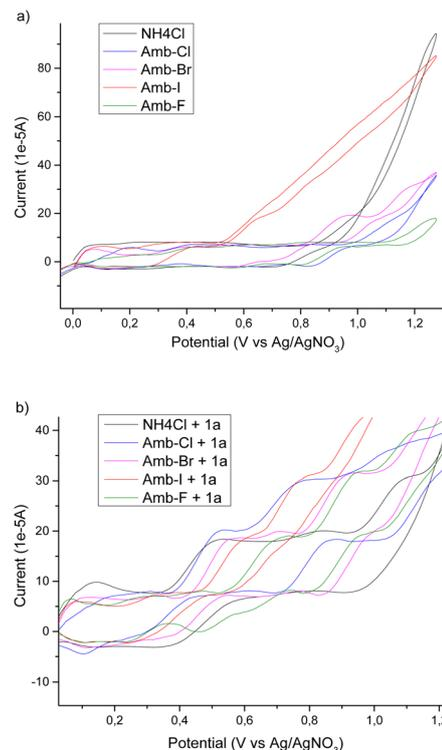
**Scheme 2** Cyclic voltammetry experiments: (a) solid electrolytes without **1a**; (b) solid electrolytes with **1a**. CV data are reported in IUPAC conventions; a glassy carbon working electrode and a platinum plated counter electrode were used with an Ag/AgNO<sub>3</sub> reference electrode filled with a 0.1 M solution of AgNO<sub>3</sub> in acetonitrile. Measurements were made at 25 °C at an initial potential of 0 V in the oxidative direction with a sweep of 100 mV s<sup>-1</sup>.
