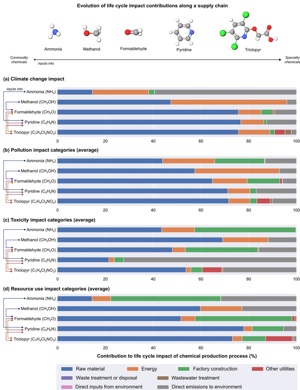
Fig. 5 Life cycle impact contribution profiles for the agrochemical product triclopyr and its precursors at various points in its upstream supply chain. Squares correspond to a feedstock materials into the process producing the indicated compound. Life cycle impact categories are grouped into four classifications – climate change, pollution, toxicity, and resource use. (a) shows contributions to climate change impacts; (b) presents contributions averaged over all pollution-related impacts (ozone depletion, particulate matter formation, ionising radiation, photochemical ozone formation, acidification, freshwater/marine/terrestrial eutrophication); (c) corresponds to average contributions to toxicity-related categories (freshwater ecotoxicity, non-carcinogenic and carcinogenic human toxicity); and (d) shows average contributions to resource use categories (land, water, minerals and metals, and fossil resource use).
