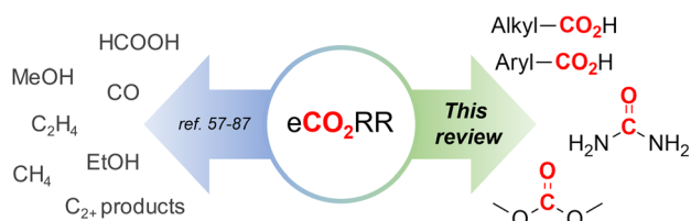
Fig. 1 Electrochemical CO 2 reduction reactions in literature and covered in this review.
