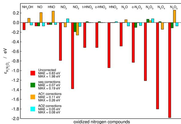
**Fig. 6** Initial and final errors in the PBE-calculated Gibbs energies of thirteen nitrogen compounds after being corrected by a chemically intuitive sequential approach (in green), an automated bond-based approach (AO1, in orange), and an automated version of the chemically intuitive, sequential approach (AO2, in cyan). Reproduced from ref. 28, licensed under CC BY 4.0 (<https://creativecommons.org/licenses/by/4.0/>).
