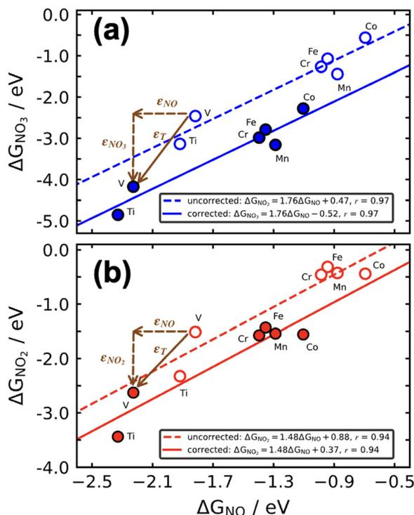
Fig. 15 Free energies of adsorption of  $^*\text{NO}_3$  (a) and  $^*\text{NO}_2$  (b) versus that of  $^*\text{NO}$  on metalloporphyrins. Dashed lines and open circles correspond to uncorrected energies, solid lines and solid circles correspond to energies upon gas-phase corrections. Brown vectors on the V-containing porphyrin show the displacements introduced by the respective gas-phase errors. Reproduced from ref. 29, licensed under CC BY 4.0 (<https://creativecommons.org/licenses/by/4.0/>).
