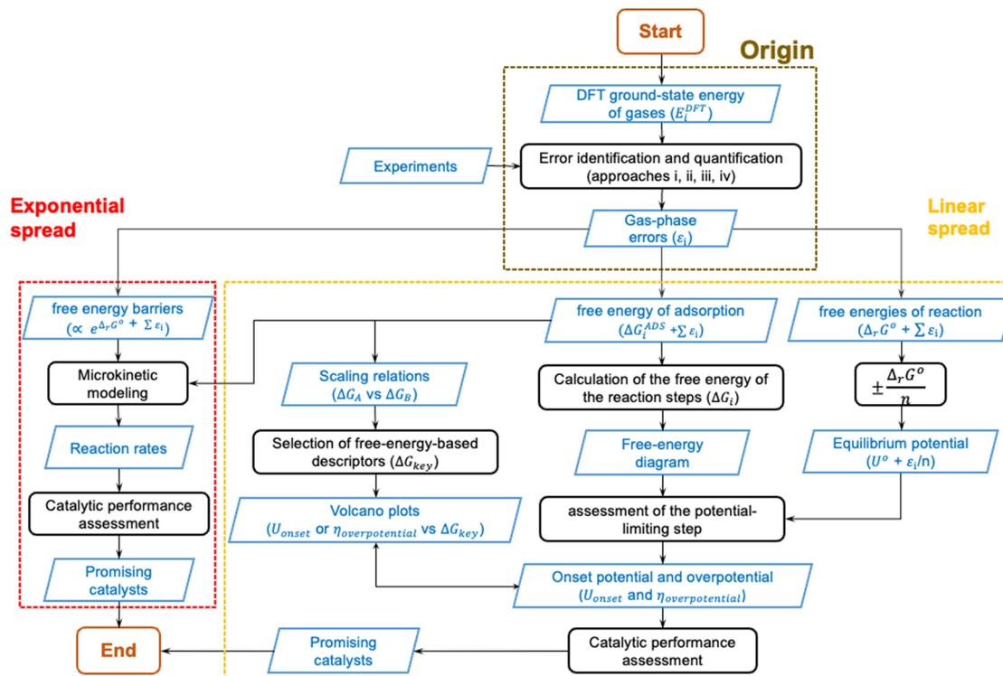
Fig. 19 Schematics of gas-phase errors ( $\epsilon_i$ ) and their impact on electrocatalysis models. The origin (brown box), exponential spread (red box), and linear spread (yellow box) in computational (electro)catalysis models are shown. Black steps represent operations performed on different datasets, depicted as blue parallelograms. Data in the blue parallelograms might lead to erroneous quantities if the errors from “Origin” are not corrected.
