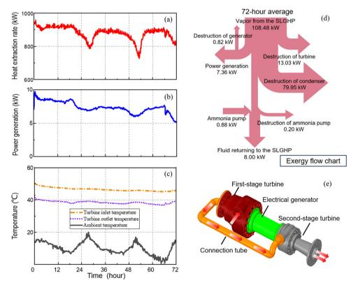
Fig. 5 Power generation performance of the SLGHP system. (a) Heat extraction rate, (b) power generation, (c) temperatures, (d) exergy flow chart, and (e) turbine structure
