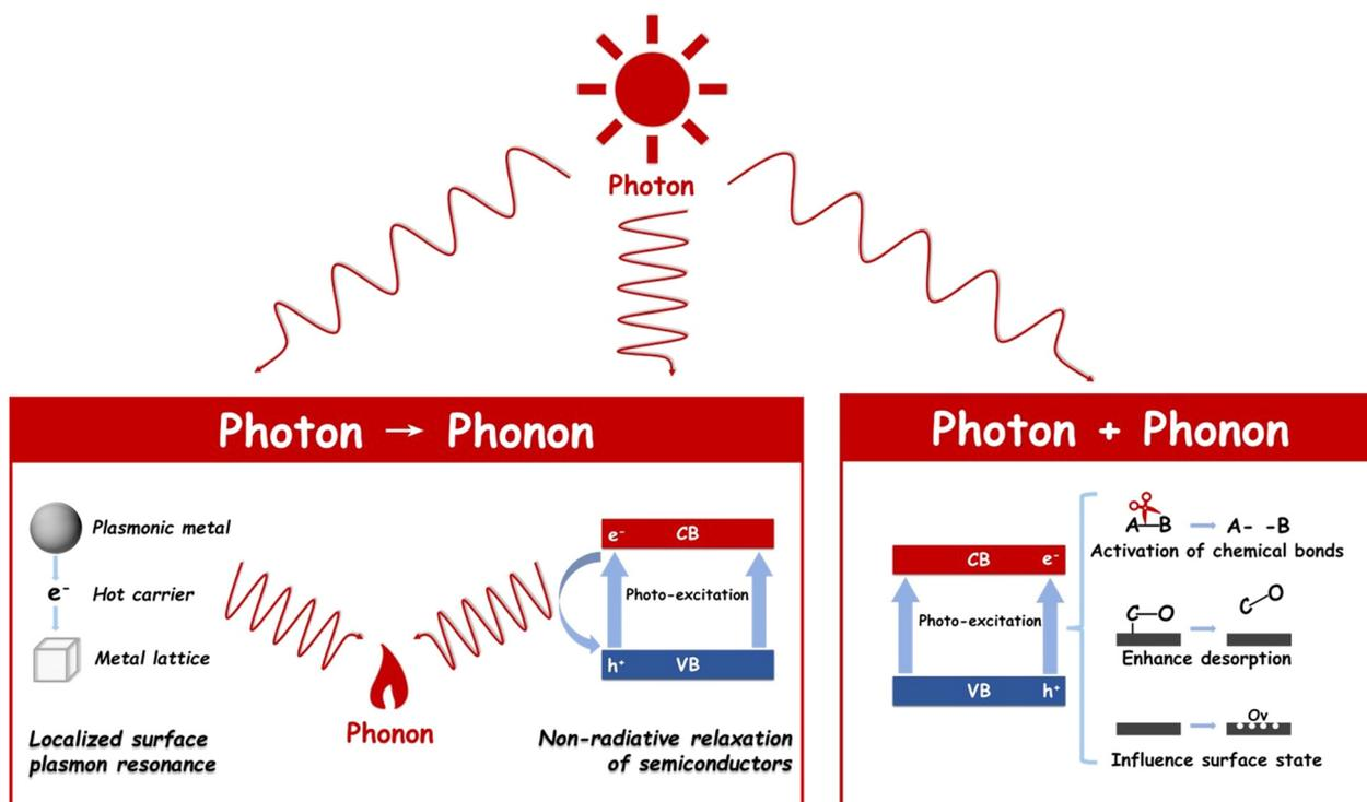
Fig. 2 Mechanism of photothermal catalysis including photons → phonons, and photons + phonons.
