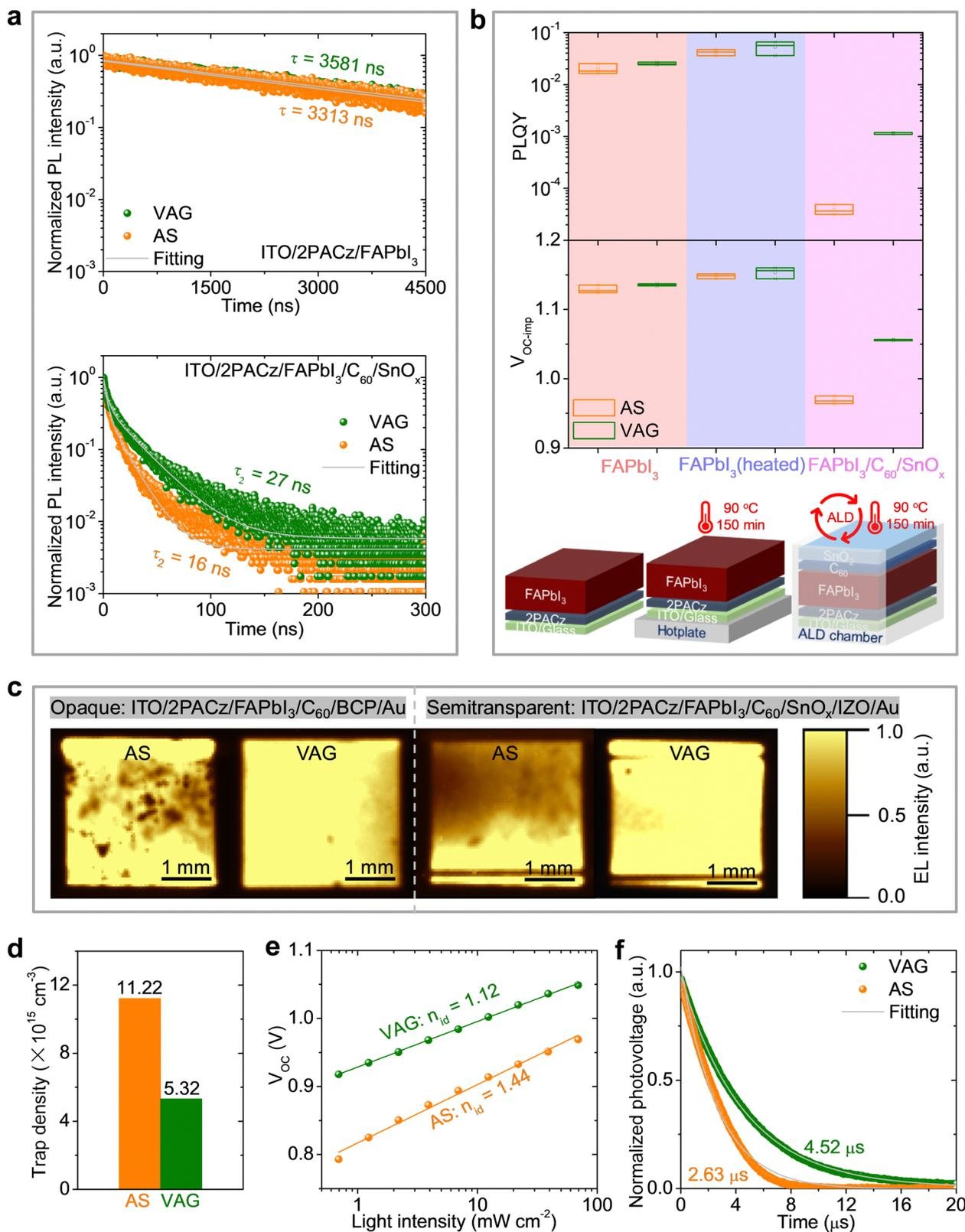
Fig. 4 Characteristics of non-radiative recombination for middle sub-cell. (a) TRPLs and (b) PLQYs for ITO/2PACz/FAPbI<sub>3</sub> and ITO/2PACz/FAPbI<sub>3</sub>/C<sub>60</sub>/SnO<sub>x</sub> stacks. (c) EL imaging of opaque and semitransparent single-junction FAPbI<sub>3</sub>-based devices. (d) Trap density obtained from the SCLC method, (e) light intensity dependence of the  $V_{OC}$ , and (f) normalized transient photovoltage decay of semitransparent FAPbI<sub>3</sub>-based devices.
