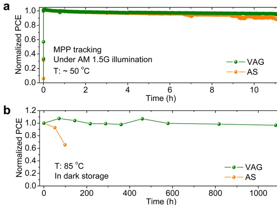
**Fig. 5** Durability of perovskite–perovskite–Si MTJSCs. Evolution of normalized PCEs of perovskite–perovskite–Si MTJSCs (a) under continuous AM 1.5G illumination at  $\sim 50$  °C for MPP tracking and (b) in dark storage at 85 °C. All devices without encapsulation were tested in an  $N_2$ -filled glovebox.
