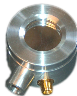
Fig. 2 Photograph of the PVDF detector with a sensitive diameter of 20 mm. On the lower left the thread for the attachment on the vertical translation stage is visible, next to it the electric connection for a 50 \Omega coaxial cable. The four detectors used in this study were custom-built by one of the authors (KL, slt@pyrosensor.de), the conductively coated foils are available on request.
