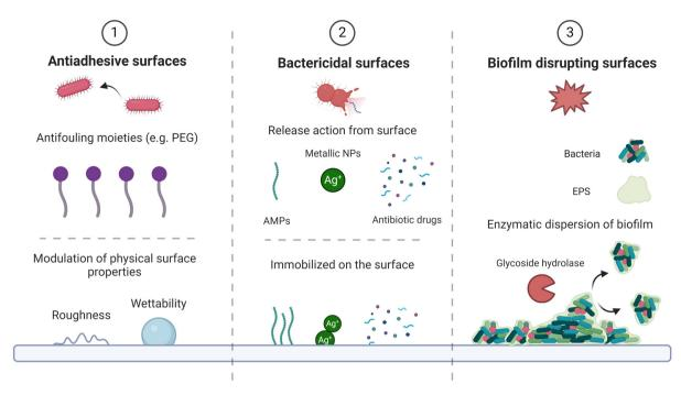
Fig. 2 Scheme summarizing the three conventional defence mechanisms adopted in the design of (1) antiadhesive surfaces, exploiting physical and chemical modifications, (2) bactericidal surfaces and (3) biofilm disrupting antimicrobial coatings, that exploit immobilization or release of active molecules. The strategies and/or molecules mentioned are a few examples of the several options available in literature.
