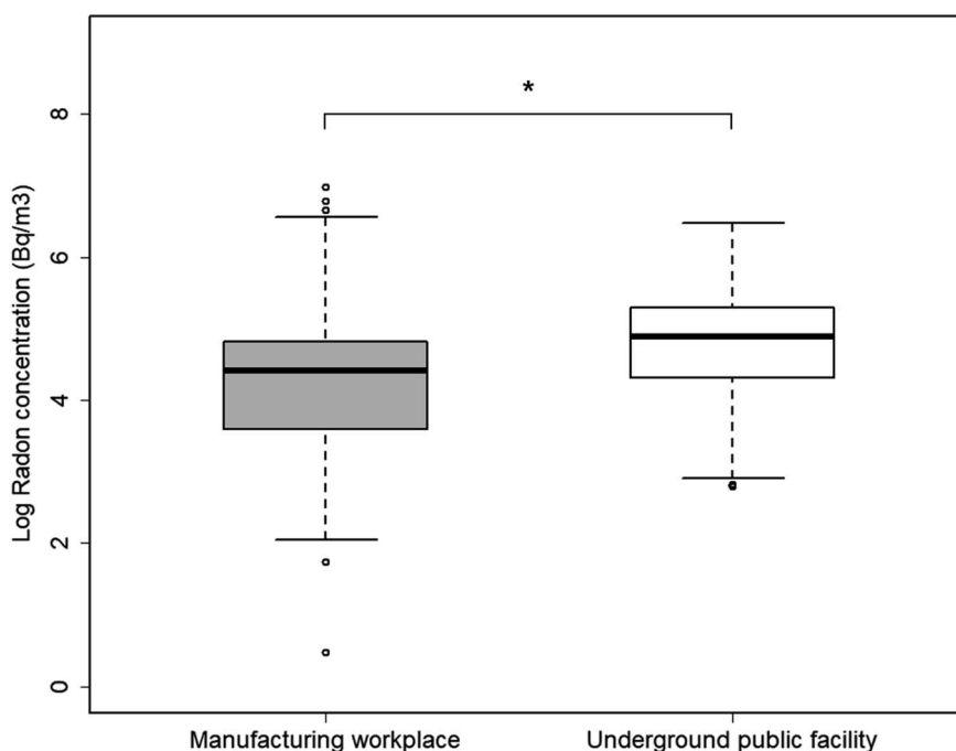
Fig. 2 Box plot of log-transformed radon concentrations measured at the manufacturing workplaces and underground public-use facilities, and the mean radon levels are significantly different ( p < 0.001 ).
