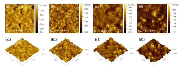
Fig. 4 AFM images. (a) 2D and (a1) 3D AFM topography images of FACs film, (b) 2D and (b1) 3D AFM topography images of FACs film with TAEA with a volumetric concentration of 200: 0.5, (c) 2D and (c1) 3D AFM topography images of FACs film with TAEA with a volumetric concentration of 200: 1, and (d) 2D and (d1) 3D AFM topography images of FACs film with TAEA with a volumetric concentration of 200:1.5.
