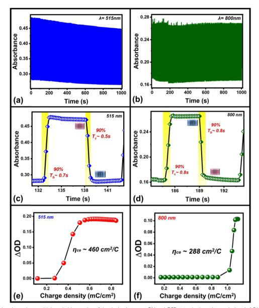
Fig. 4 (a) In situ bias-dependent multiple switching cycles of the device between ON and OFF states in the voltage window (±1.5 V) in the visible and infrared (IR) wavelength region in (b) and (c) single switching cycle at 515 nm wavelength, (d) response time of the device in the same fixed voltage window at 800 nm wavelength, and the corresponding estimated coloration efficiencies of the device in (e) and (f).
